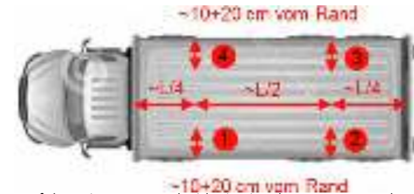
Fig. 3: Diagram of the points measured with piercing thermometer on the trucks
