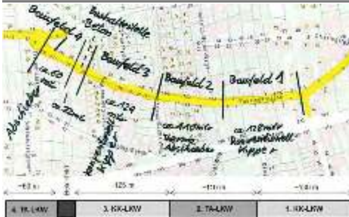
Fig. 1: Layout of the four construction plots
