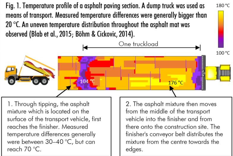
1. Through tipping, the asphalt mixture which is located on the surface of the transport vehicle, first reaches the finisher. Measured temperature differences were between 30–40 °C, but can reach 70 °C.
