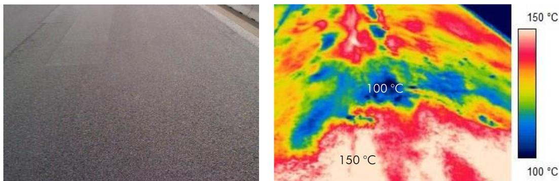
Fig. 3 (le) and 4 (ri): Normal photography and temperature profile taken with a infrared camera (Photo: Rošer, 2020).
