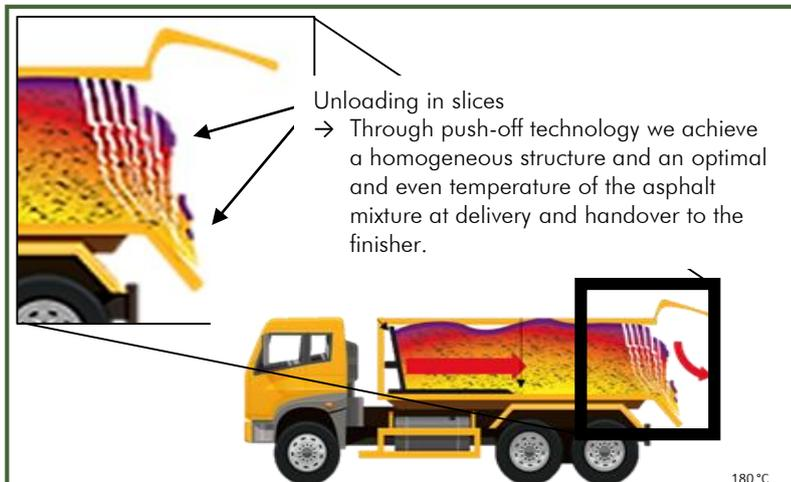
Fig. 5: Transport vehicle with push-off technology for delivering asphalt mixtures (Illustration: EPA).
