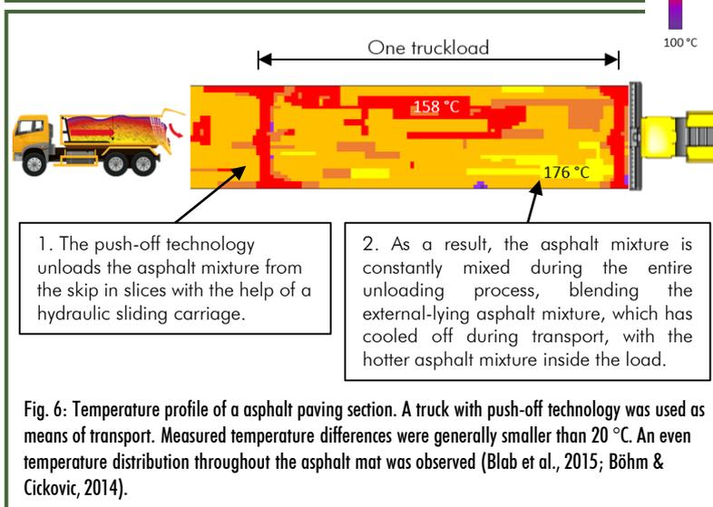
Fig. 6: Temperature profile of an asphalt paving section. A truck with push-off technology was used as means of transport. Measured temperature differences were generally smaller than 20 °C. An even temperature distribution throughout the asphalt mat was observed (Blab et al., 2015; Böhm & Cickovic, 2014).
