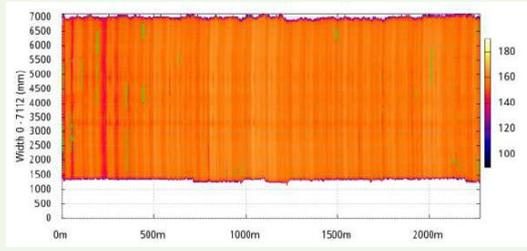
Fig. 8: Surface temperature profile with infrared camera (SBUFb, 2018).
